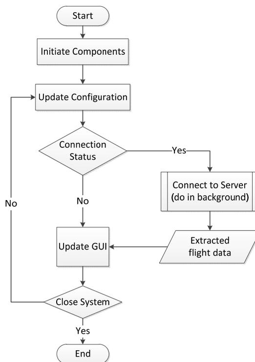
Fig. 1 The main workflow of Ground System Software
