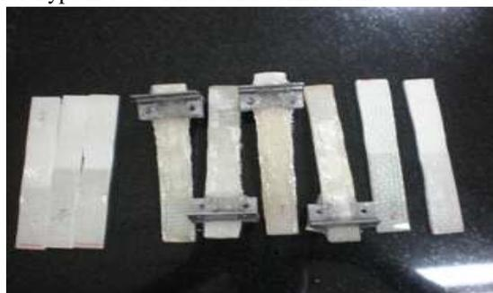
Fig. 3 Specimens for both DCB Test and ENF Test
