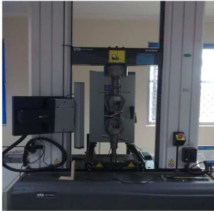
Fig. 4 Experimental set up for DCB Test
