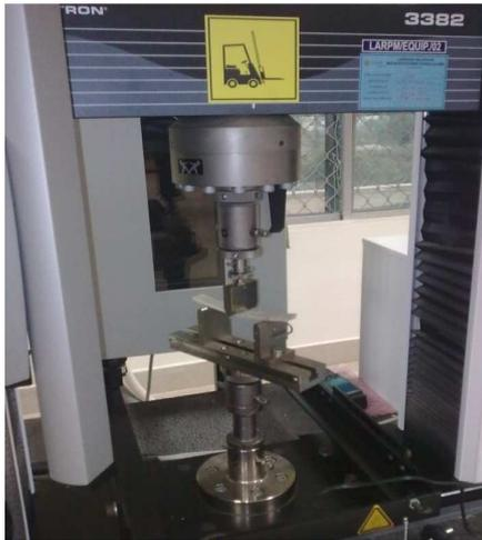
Fig. 5 Experimental setup for ENF Test
