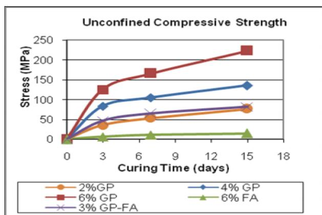
Fig. 6. UCS of treated and untreated soil
