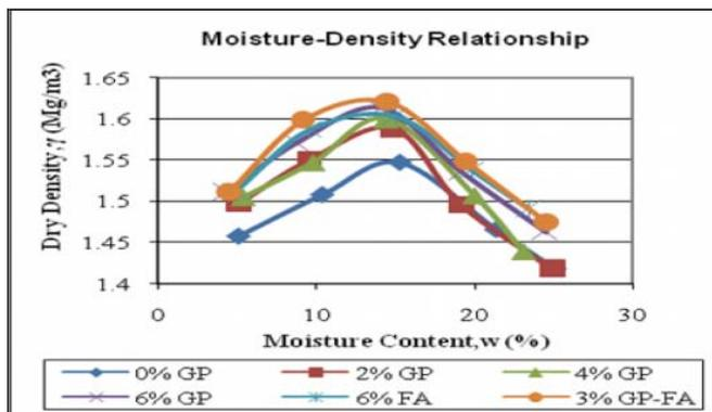
Fig. 3 Compaction curve of treated and untreated soil
