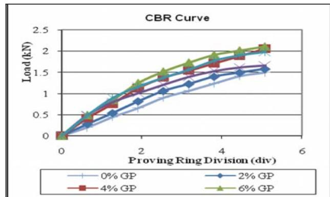
Fig. 4 CBR of treated and untreated soil
