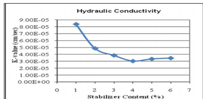
Fig. 5 Permeability of treated and untreated soil.
