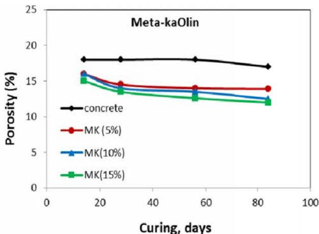
Fig. 3 Porosity decrease of specimens during concrete curing
