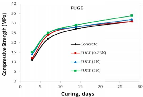
Fig. 6 Strength Measurement on FUGE chemical on a 28 days period
