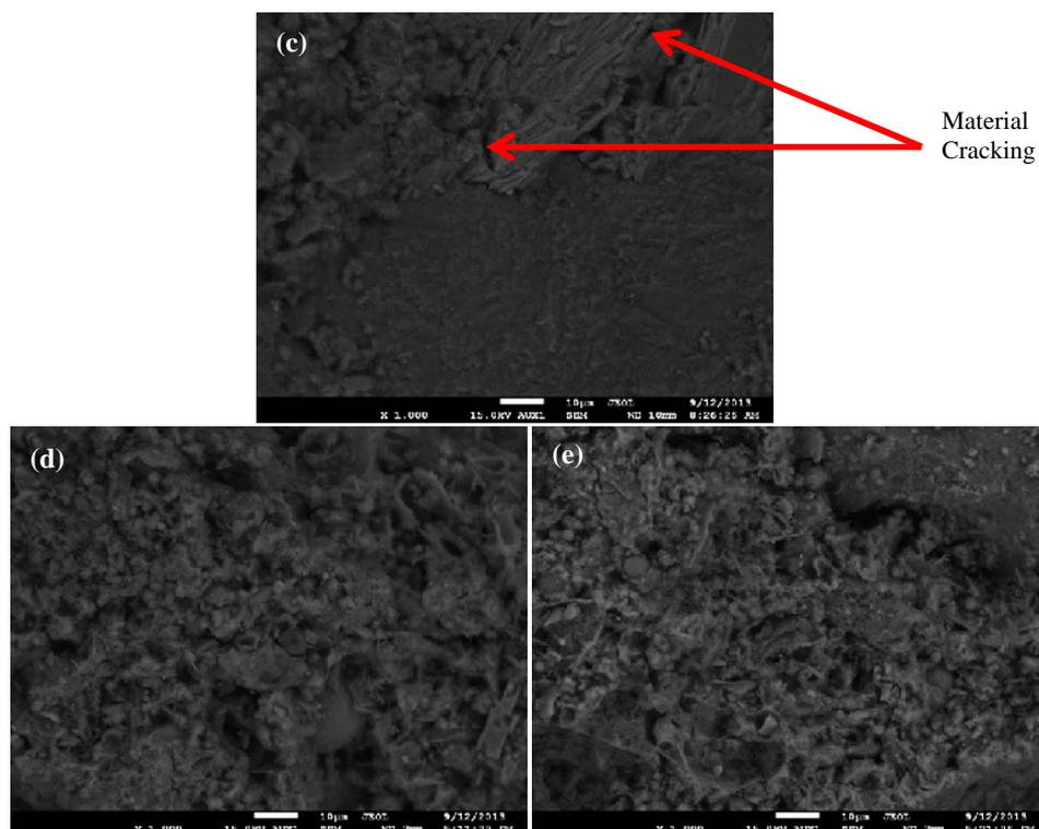
Fig. 9 Scanning Electronic Microscope (SEM) results control mortar and chemical admixtures (c) control mix, (d) FUGE and (e) Borax solution (1000x) after 84 days of curing
