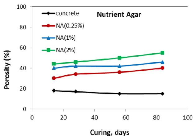
Fig. 2 Porosity increase of specimens during concrete curing
