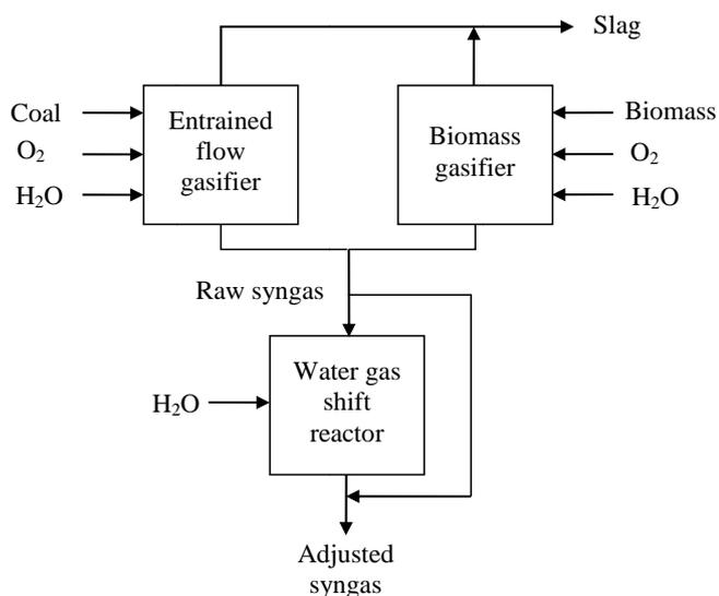
Fig. 2 Schematic diagram for independent co-gasification process
